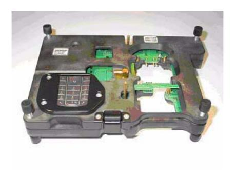
Note: The supply voltage for the MJ-12 has to be kept within the range of 8-12 V when using the built in regulator. When bypassing the regulator (IMEI rewrite), the voltage must be kept below 5,4V.
